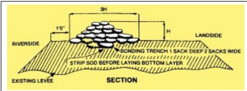
Place the sandbags to form a pyramid by alternating header courses (bags placed crosswise) and stretcher courses (bags placed lengthwise).
